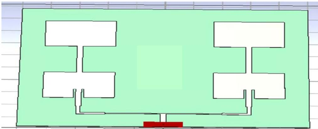
Figure 8: 2 x 2 cooperate-series-fed 2 x 2 MSA array designed in CST studio.
