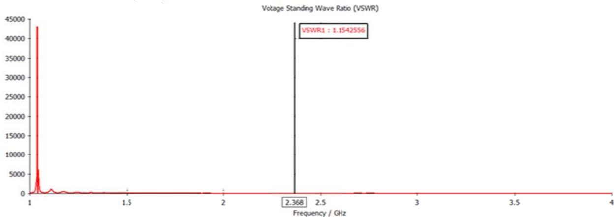
Figure 12: VSWR of 1 x 2 cooperate antenna array at 2.4 GHz.
