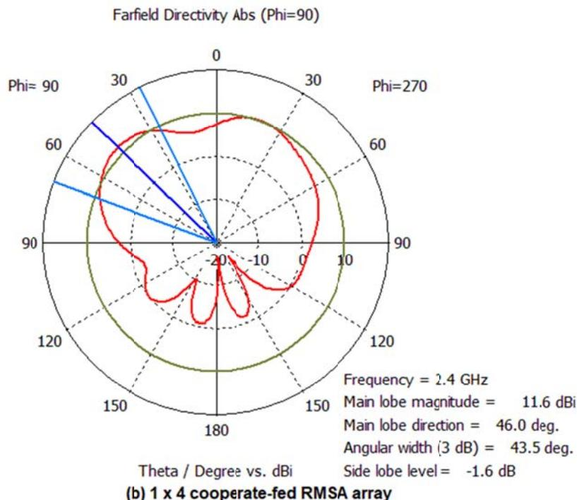
Figure 15: Directivity of the 1 x 4 cooperate-fed antenna arrays at 2.4 GHz in H-plane ( $\varphi = 90^\circ$ ).
