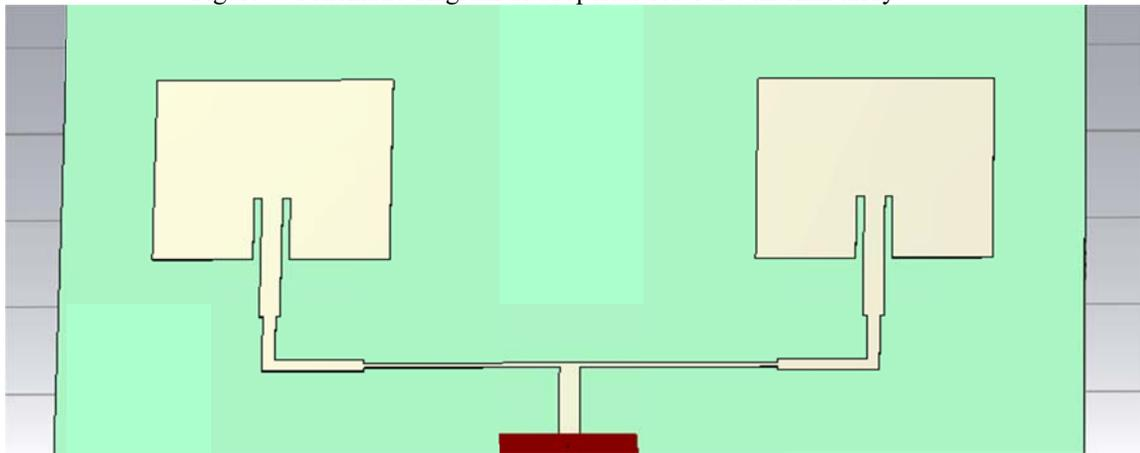
Figure 5: 1 x 2 cooperate-fed MSA array designed in CST studio.
