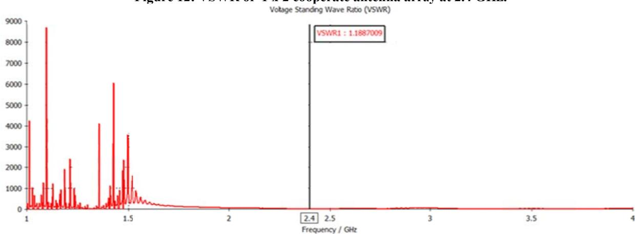
Figure 13: VSWR of 1 x 4 cooperate antenna array at 2.4 GHz.
