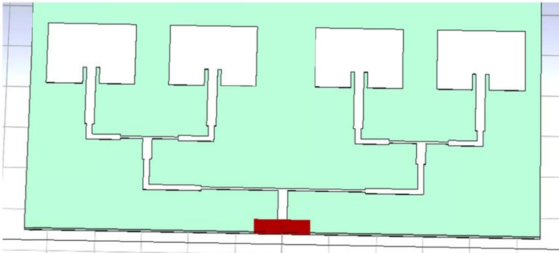
Figure 6: 1 x 4 cooperate-fed MSA array designed in CST studio.
