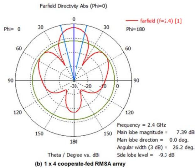
Figure 17: Directivity of array antennas at 2.4 GHz in E-plane ( $\phi = 0^\circ$ ).
