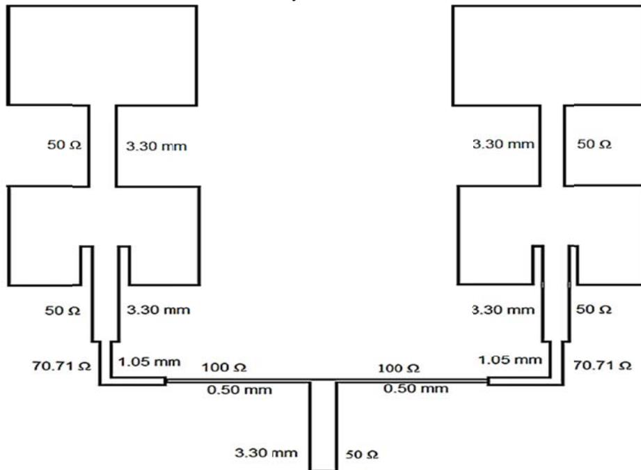
Figure 7: Schematic diagram of cooperate-series-fed 2 x 2 antenna array.
