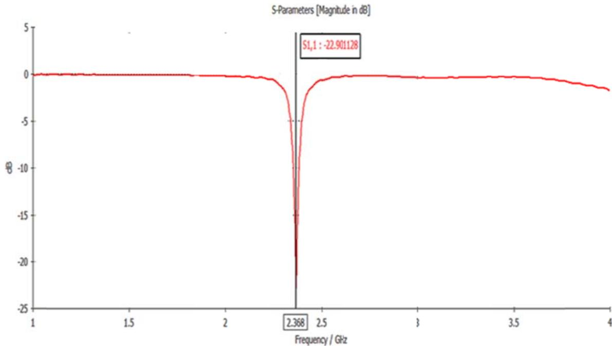
Figure 9: Return loss plot of the 1 x 2 cooperate-fed antenna array.
