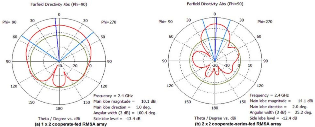
Figure 16: Directivity of antenna arrays 1 x 2 cooperate-fed and 2x2 cooperate-series-fed RMSA array at 2.4 GHz in H-plane ( $\phi = 90^\circ$ ).
