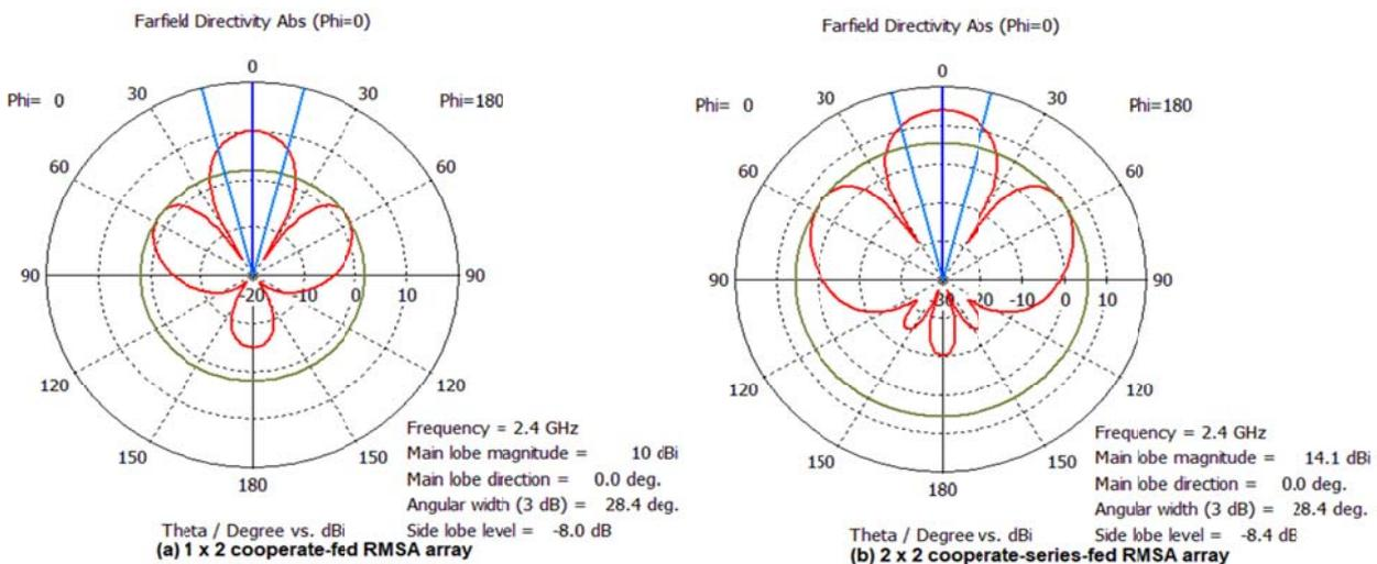
Figure 18: Directivity of array antennas at 2.4 GHz in E-plane ( $\phi = 0^\circ$ ).
