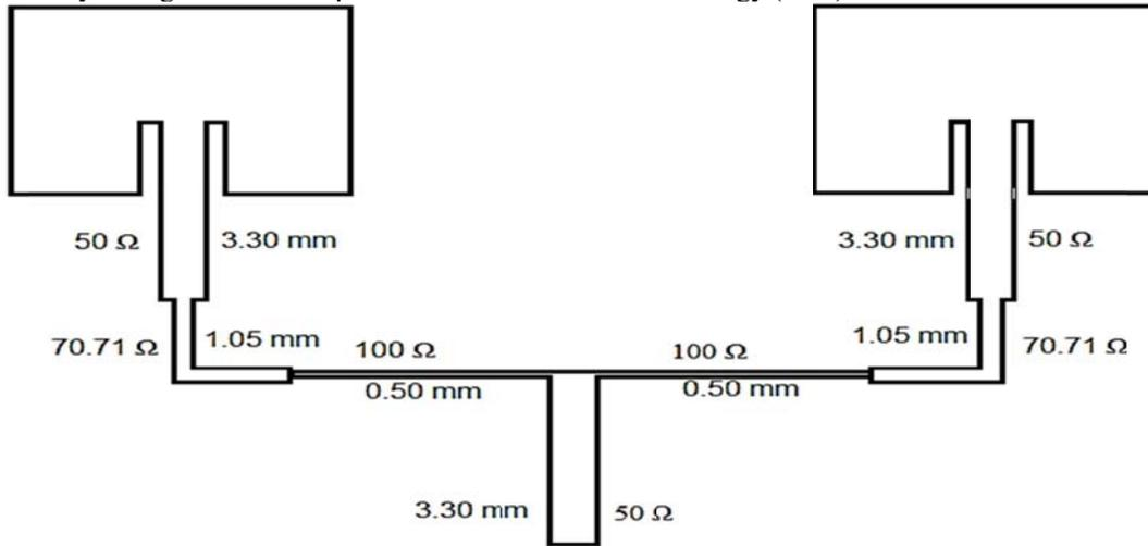
Figure 3: Schematic diagram of cooperate-fed 1 x 2 antenna array.
