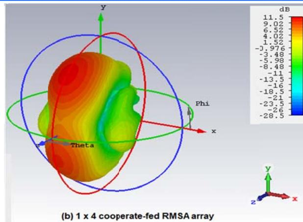
Figure 19: The 3-D gain of the 1 x 4 cooperate-fed RMSA array at 2.4 GHz.
