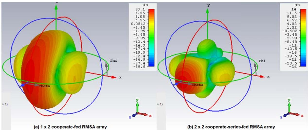
Figure 20: The 3-D gain of the 1 x 2 cooperate-fed and the 2 x 2 cooperate-series-fed RMSA array at 2.4 GHz.
