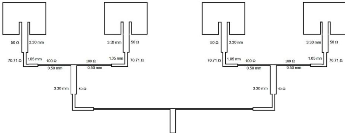
Figure 4: Schematic diagram of cooperate-fed 1 x 4 antenna array.
