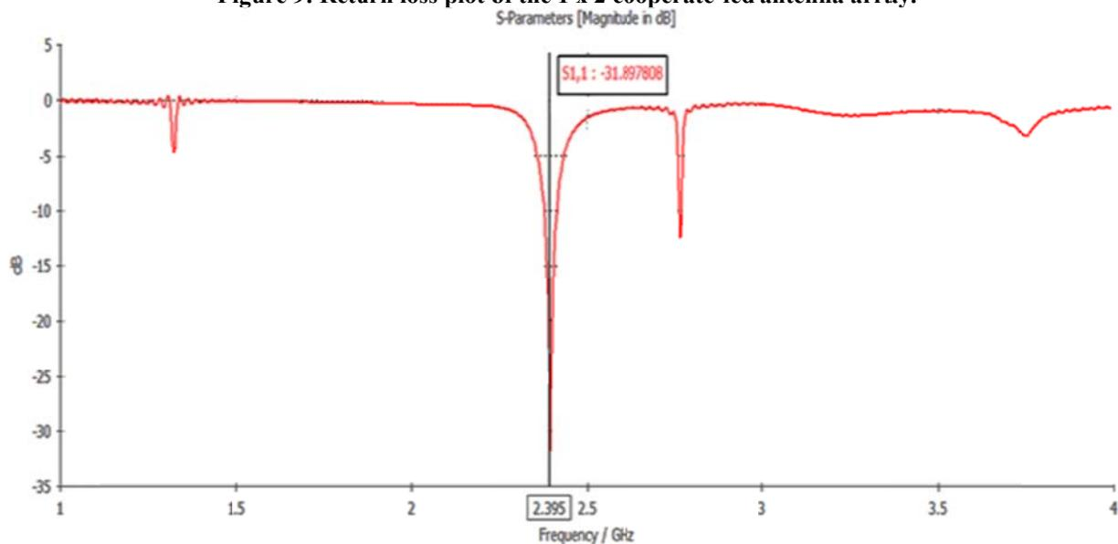
Figure 10: Return loss plot of the 1 x 4 cooperate-fed antenna array.
