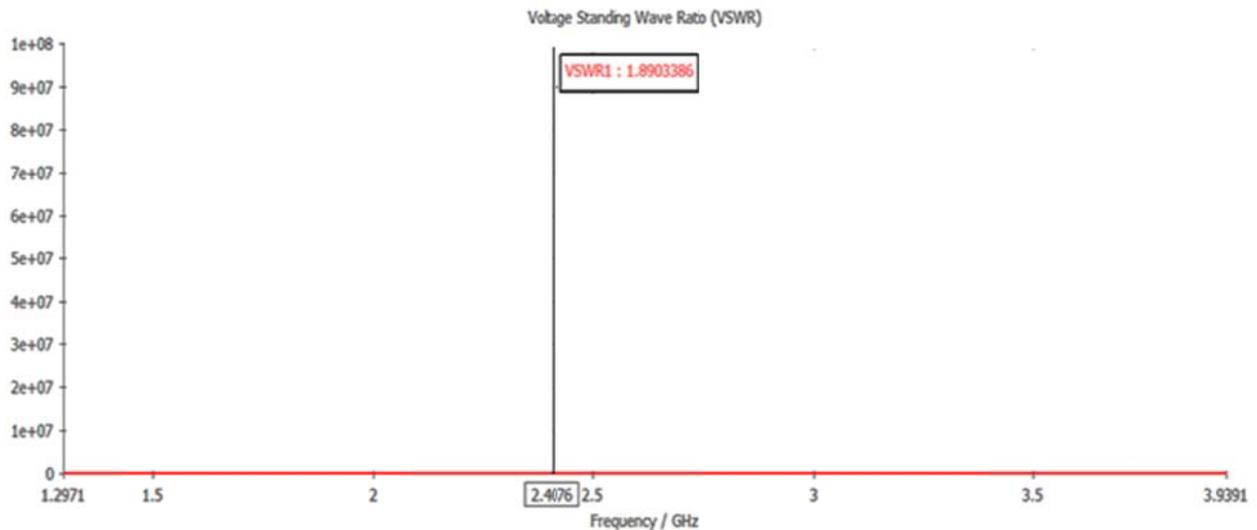
Figure 14: VSWR of 2 x 2 cooperate-series-fed antenna array at 2.4 GHz.
