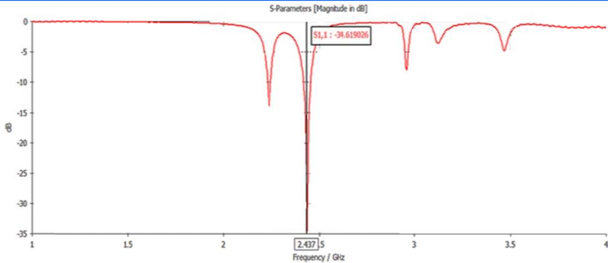
Figure 11: Return loss plot of the 2 x 2 cooperate-series-fed antenna array.
