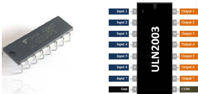
Figure 12: ULN2003 IC for driving the relay and its Pin-out
