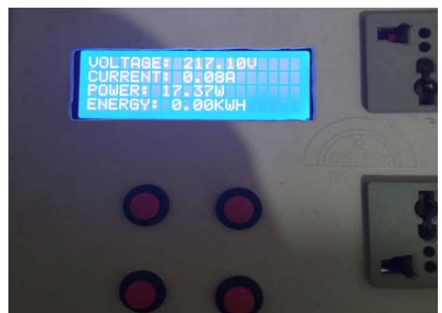
A. Figure 17 Output interface showing the screen display and the socket outlets
