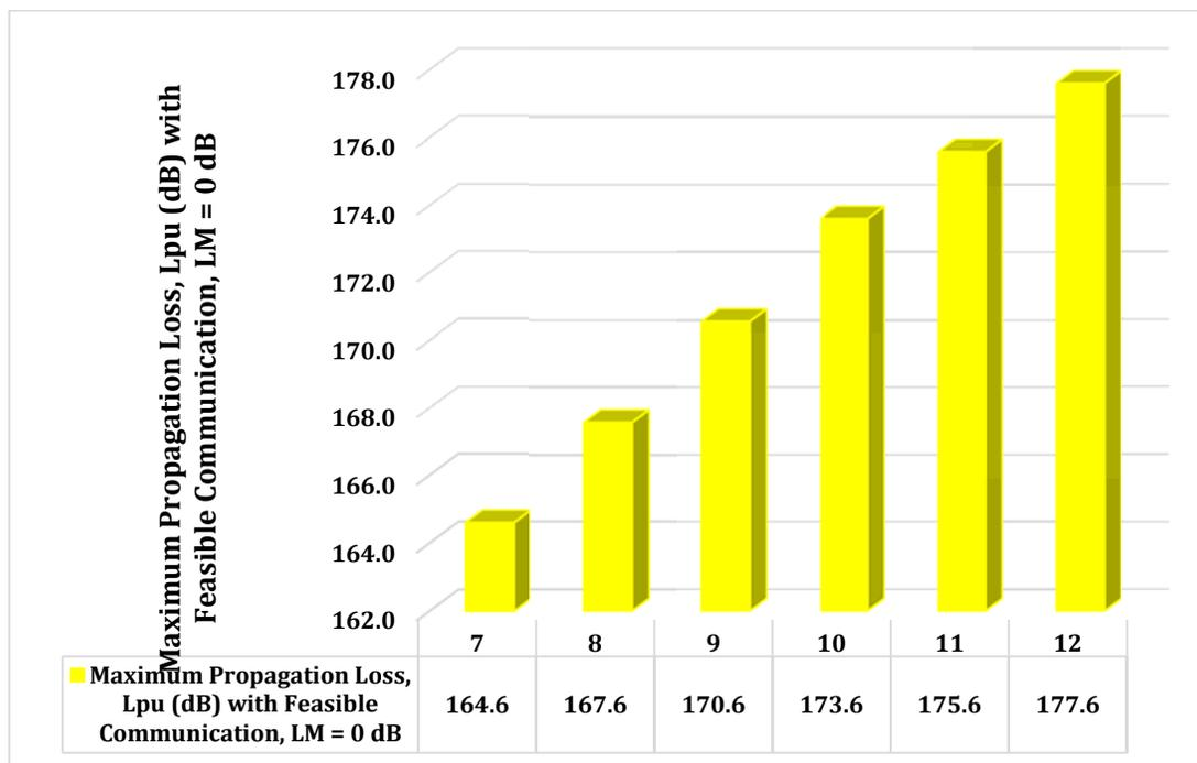
Figure 6 The bar chart of the maximum propagation loss supported for the satellite link with feasible network communication for the five different spreading factors, SF , SF , SF operated in LoRa transceivers
