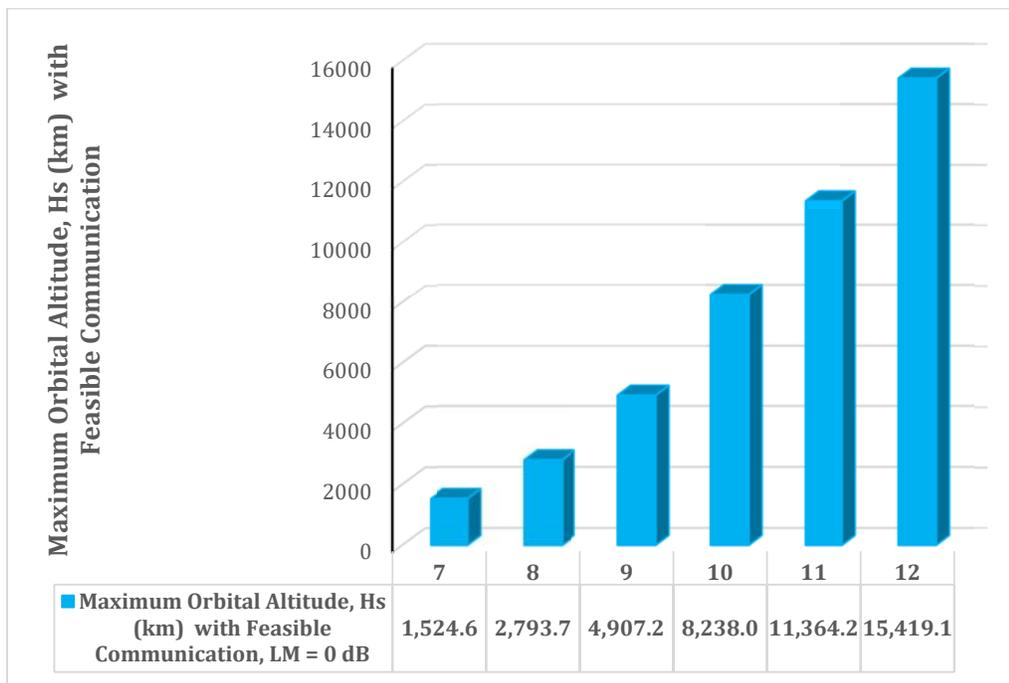
Figure 2 The bar chart of the maximum orbital altitude of the satellites with feasible network communication for the five different spreading factors, SF , SF operated in LoRa transceivers
