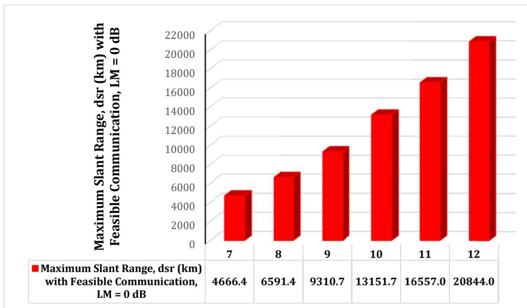
Figure 4 The bar chart of the maximum slant range of the satellites with feasible network communication for the five different spreading factors, SF , SF operated in LoRa transceivers
