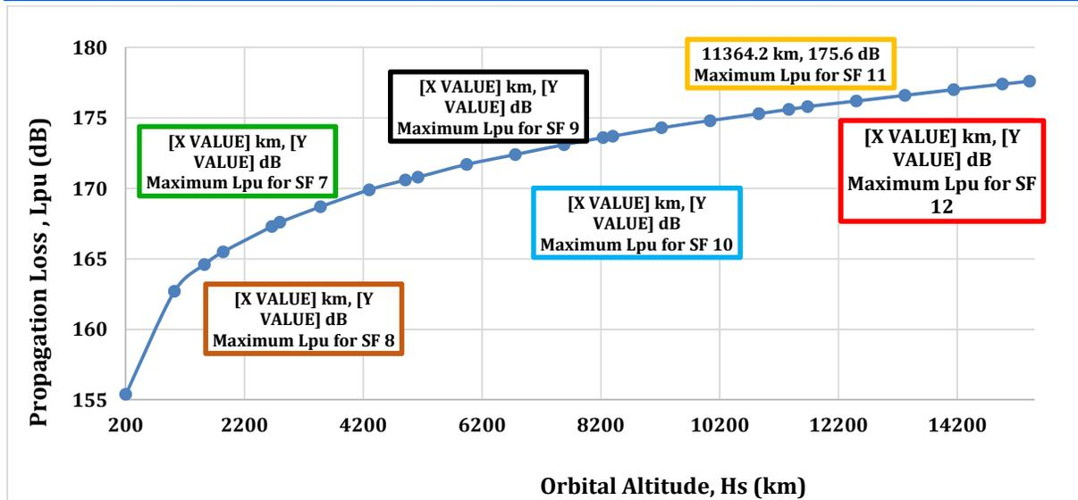
Figure 5 The graph of the propagation loss versus orbital altitude of the satellites for the five different spreading factors, SF , SF operated in LoRa transceivers.
