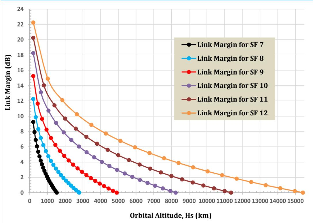
Figure 1 The graph of the link margin versus orbital altitude of the satellites for the five different spreading factors, SF , SF operated in LoRa transceivers.
