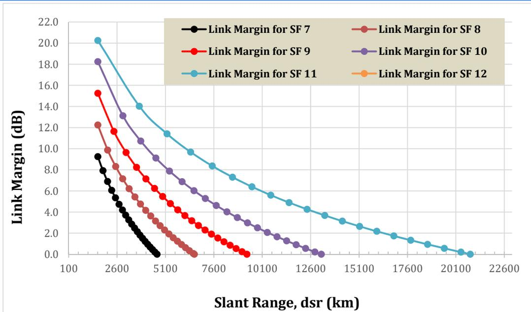
Figure 3 The graph of the link margin versus slant range of the satellites for the five different spreading factors, SF , SF , SF operated in LoRa transceivers.
