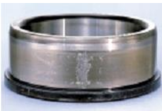
b. Pitting on the inner rings in cylindrical ball bearings
