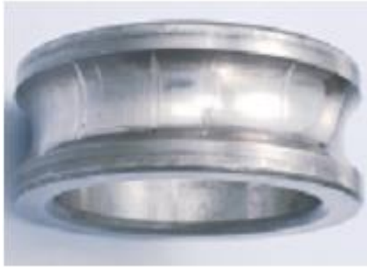
e. Wear by friction with the inner ring of the roller bearings Figure 6. Some pictures of wear of the bearings
