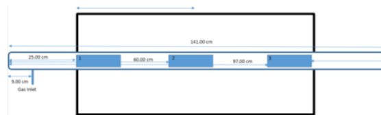
Figure 2. Schematic distribution of the position of the stainless steel container for MWCNTs synthesis.
