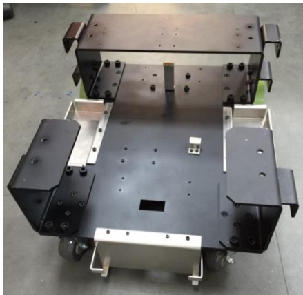
Fig. 6. Photo of AGV frame.
